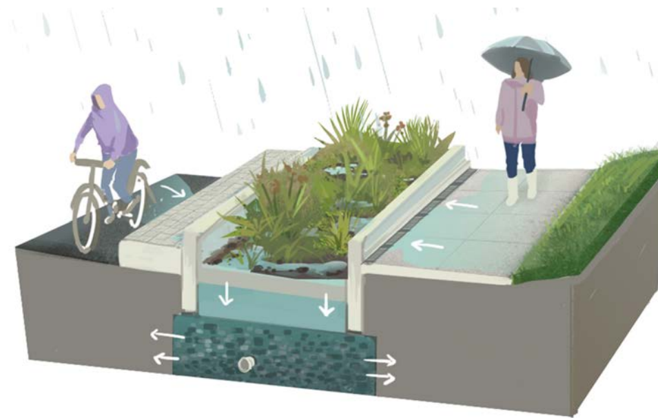
Figure 101. Permeable paving and bioswales help filter contaminants out of the stormwater running into Valley Creek and the Strait of Juan de Fuca
